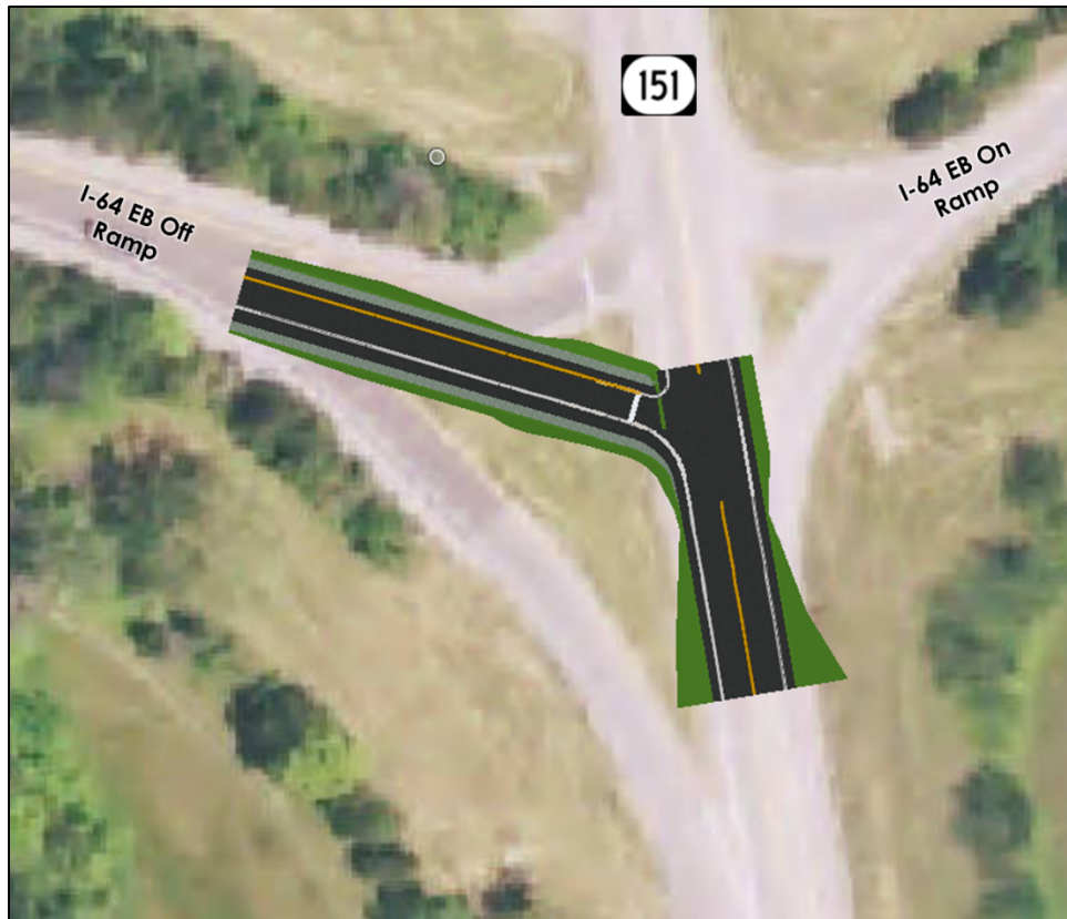
Figure 7: Realignment of I-64 EB off ramps
